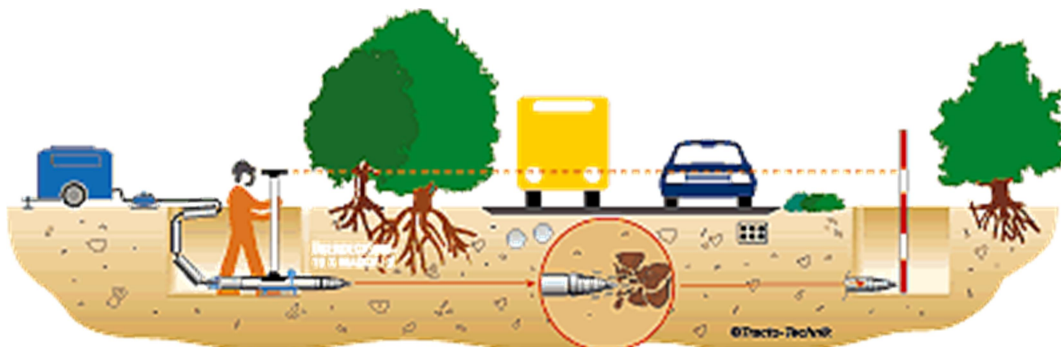
Figure 18: Image of Trenchless Technology for Installation of Cable
